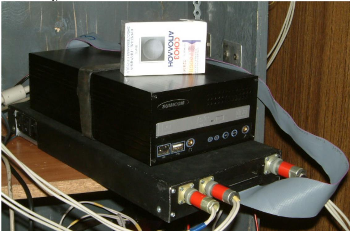
View of interface connected to data acquisition board (16 bit NI DAQ) installed in industrial computer.
