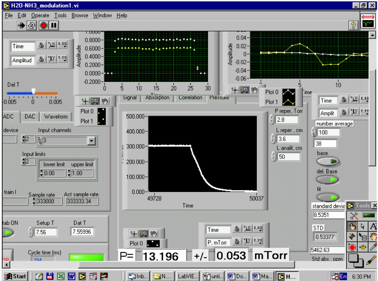
A view of software control panel during purification process. Central screen shows a decrease of water.
