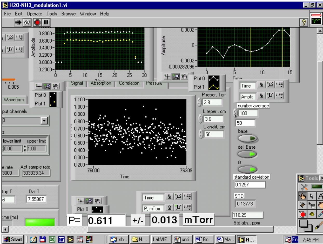
Central screen shows water concentration in ammonia in mTorr (partial water vapor pressure). Ammonia pressure in this experiment was 21 Torr. Standard deviation of 0,013 mTorr corresponds to 2.5 ppm for 0.3 sec averaging time.
