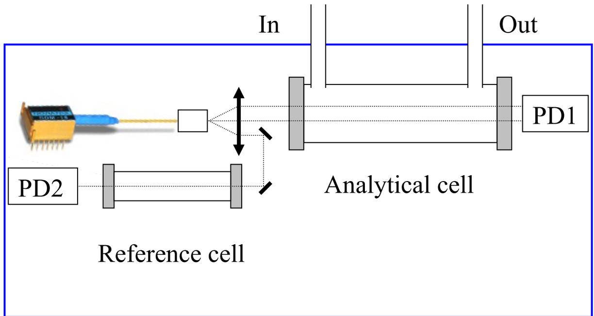
Fiber output laser radiation was collimated by a lens into nearly parallel beam. Small part of radiation (approximately 5 %) was sent to reference channel, passed sealed reference cell 36 mm long with 1.9 Torr of water vapor. Analytic channel incorporated 0.5 m long 40 mm diameter electropolished stainless steel tube with glass windows.
