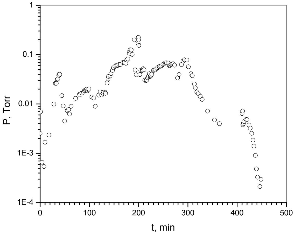
Example of water continuous monitoring during the process of ammonia purification. The lower outlet of column, having the excess of water was investigated. During the process under consideration its parameters were optimized based on data obtained (details will be published elsewhere). Results presented on Fig. shows that optimized purification process can be finished after 450 min. This time is significantly less than it was considered traditionally.
