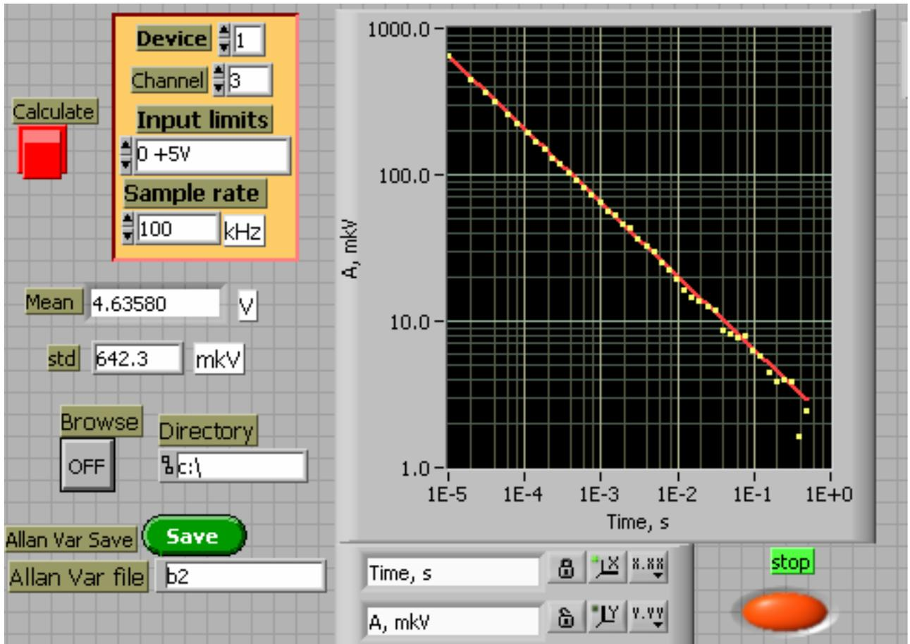
Allan deviation of signal in analytic channel. In present case minimum detectable absorption was determined by resolution of 12 bit NI data acquisition board and corresponds to  $10^{-6}$  for 0.1 sec averaging time.
