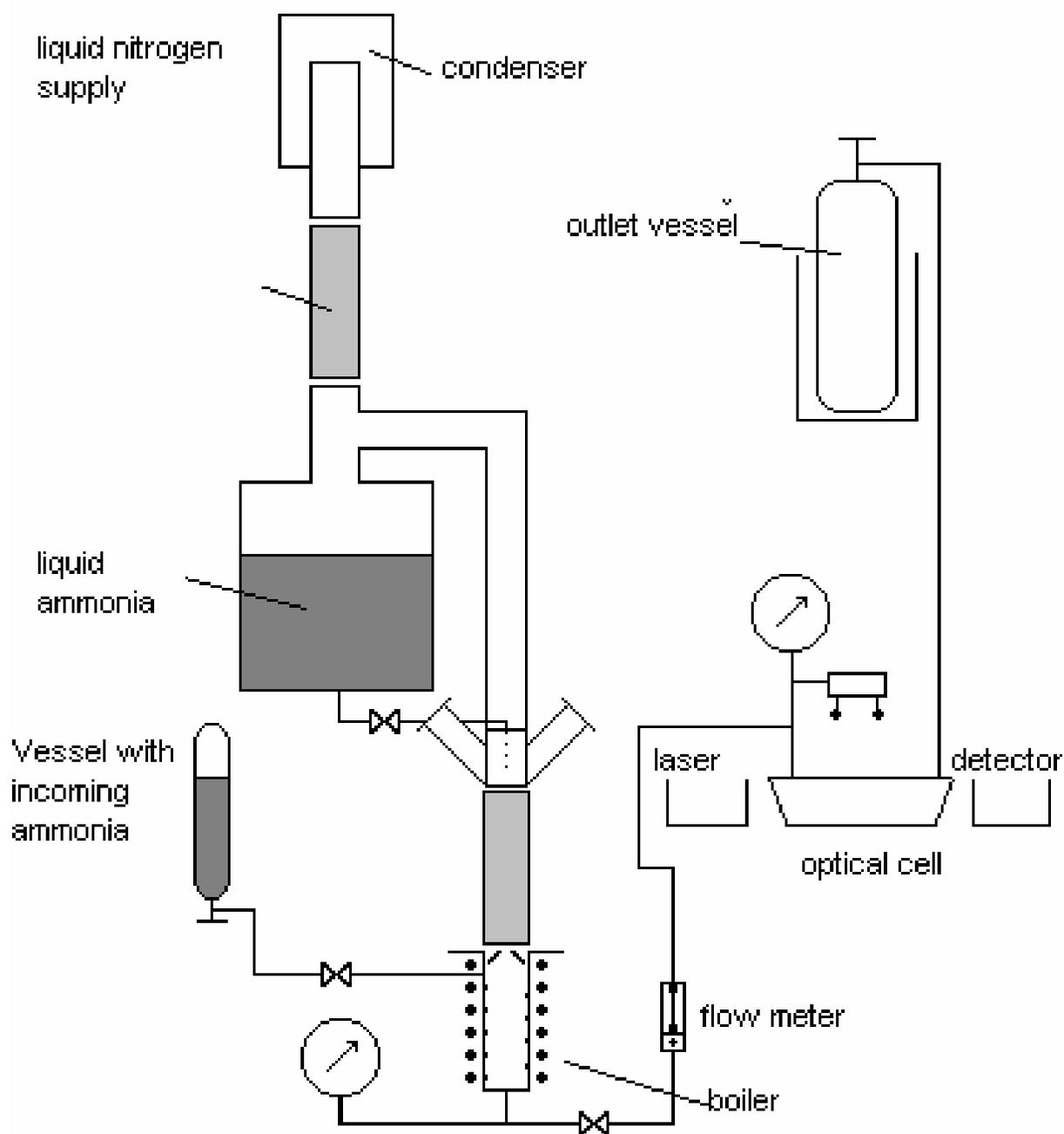
Block scheme of purification column and the instrument installation
