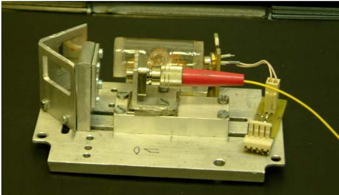
View of optical elements with reference cell
