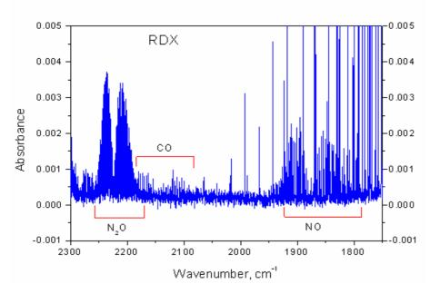
Absorption spectra (FTS Bruker 66-v) of explosives decomposition products have been investingated using FTS Bruker 66-v.
