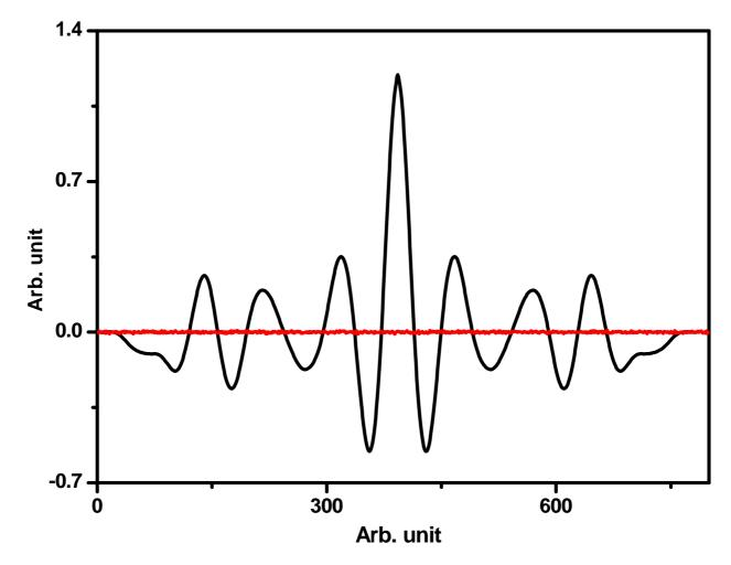
Autocorrelation function of reference signal (black) and crosscorrelation function of analytical and reference signals (red).
