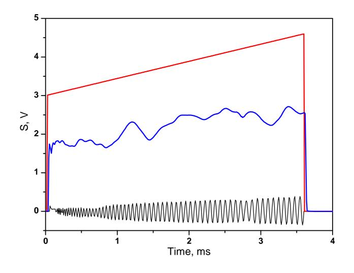
Recorded signals in analytical (red) and reference (blue) channels when laser was excited by trapezoidal periodical current pulses. Black line shows FP etalon fringes for frequency scale calibration (0.05 cm<sup>-1</sup> free spectral range). For convenience long pulse is presented. In experiment pulse duration was 0.12-0.4 ms.
