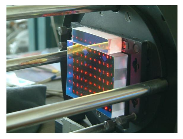
Multipass cell: baselength - O.5 m, dielectric mirrows with 99.9 % reflectivity; 282 passes, 141 m.
