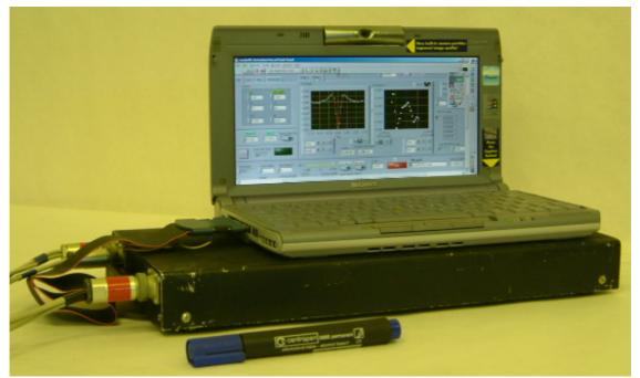
View of interface connected to data acquisition board (12 bit NI DAQ) installed in notebook.
