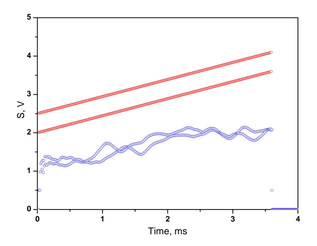
Recorded signals in analytical (red) and reference (blue) channels when modulation was added to excitation current. It looks like two frequency laser operation with tuning (see separate poster). Then difference signal between two branches can be calculated. For convenience long pulse is presented. In experiment pulse duration was 0.12-0.4 ms.
