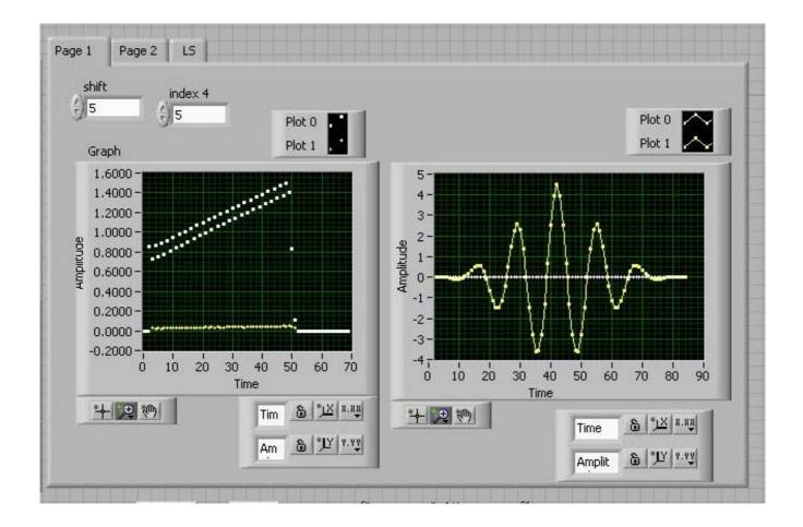
Software developed control panel. Left picture – analytical (white) and reference (yellow) signals. Right picture – correlation functions of analytical (white) and reference (yellow) difference signals (see above).
