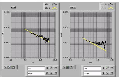
Software control panel to measure Allan deviation in two independent channels (in present case analytical signal and temperature).
