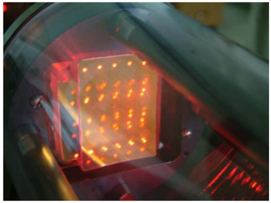
Multipass cell: baselength - 25 cm, dielectric mirrows with 99.5 % reflectivity; 132 passes, 33 m.
