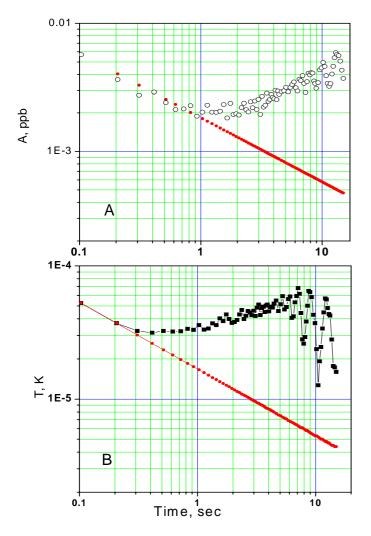
Allan deviation of minimum detectable NO<sub>2</sub> concentration (A) and temperature (B). Concentration was measured at atmosphere pressure and minimum detectable absorption was found to be 2.7 ppt (atmosphere pressure broadened spectrum) and 0.75 ppt for reduced pressure (broadening is close to Doppler one).
