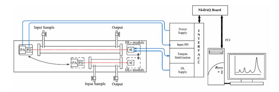
Distributed feedback (DFB) diode laser (DL) from Laser Components GmbH was used. The wavelength of lasing was in the vicinity of 1.392  $\mu$ . The DL was pumped with trapezoidal pulses of 0.5–1 ms duration and 1–2 kHz repetition rate. Frequency tuning of the DL radiation was produced in the frequency interval 7183.2–7185.0 cm<sup>-1</sup>.
