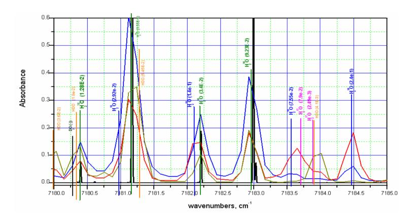
Absorption spectra of water vapor with different isotope contents as recorded with the Fourier-spectrometer with the 0.025 cm<sup>-1</sup> spectral resolution. In brackets absorption line cross-sections (cm<sup>-2</sup>/atm) are presented [1,2]. The frequency range of 7182.5-7185 cm<sup>-1</sup> was chosen for simultaneous measurement of the following isotopomers:  $H_2^{16}O$ ,  $H_2^{17}O$ ,  $H_2^{18}O$ ,  $HD^{16}O$ ,  $D_2^{16}O$ .
