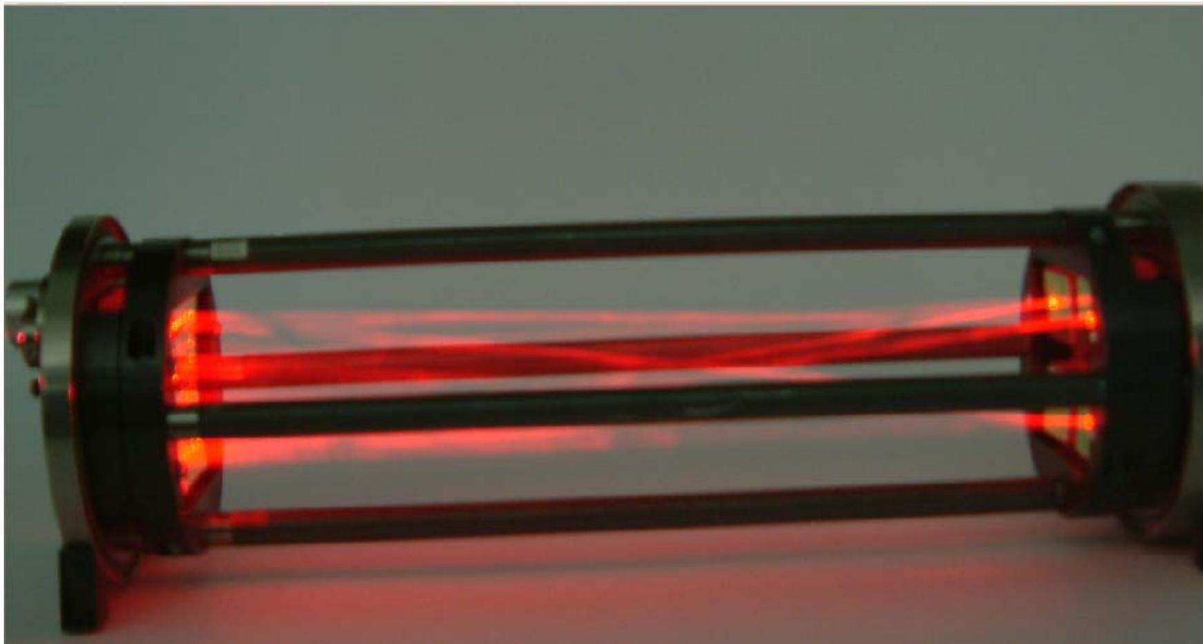
Fig. 1 View of Chernin matrix multipass cell, 25 cm base length, 156 passes.
