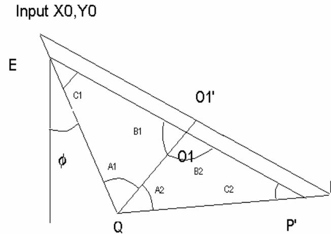
Details of calculation: position of incoming beam on spherical mirror was calculated using stereometric task solution, using projection of a beam reflection on a base X-Y plane. Position of a beam on mirror surface was found as mutual solution for a given sphere surface equation and linear X-Y projection on base surface equation.
