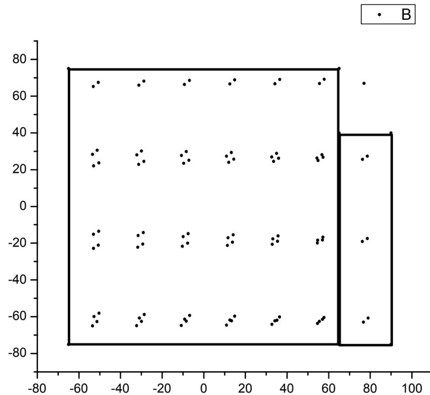
Experimental and calculated matrix of images on field mirrors (two sets of mirrors were separated from ideal position by 2.8 mm)
