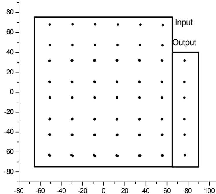
Experimental and calculated pattern of images on fields mirrors for the cell with 1200 mm mirrors curvature. The picture was obtained with parallel beam of He-Ne laser. As could be seen, pairs of images in ideal matrix do not fully coincide – this is due to final distance between two sets mirrors. The same effect leads to aberrations.
