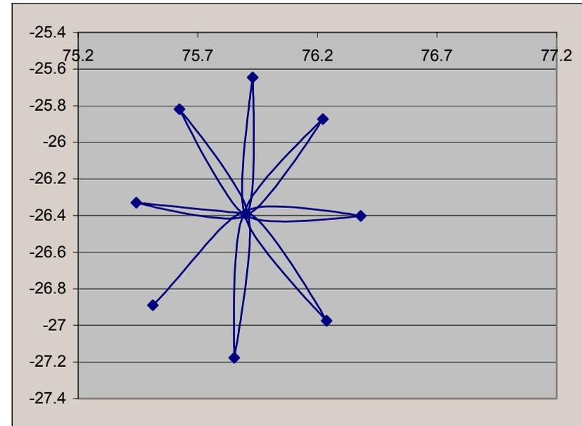
Aberrations were calculated as a middle distance between center and peripheral aberration spot frame. Minimal experimentally observed output aberration was 8 mm.
