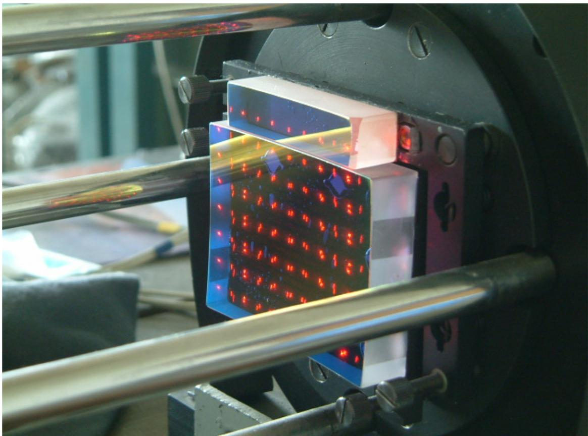
Multipass cell: baselength - 0.5 m, dielectric mirrors with 99.9 % reflectivity; 282 passes, 141 m.
