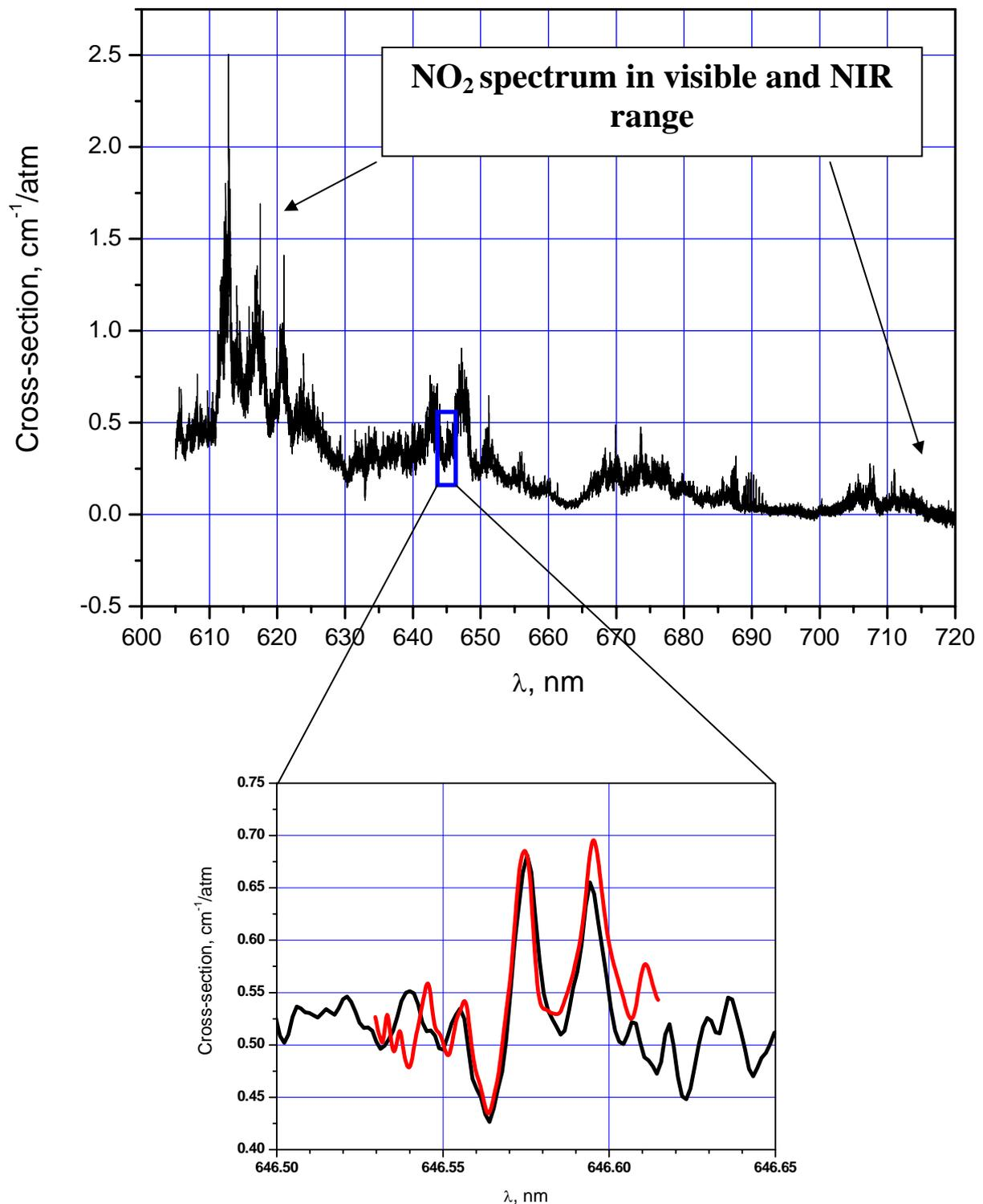
**Identification of the Diode Laser and FT spectra near 646 nm. The Diode lasers that have been tested included about 70 visible (635-680-nm) diode lasers manufactured by Toshiba, Sanyo, Hitachi, Mitsubishi and Russian companies (Polus, Nolatech).**
