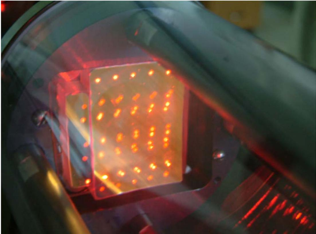
Multipass cell: baselength - 25 cm, dielectric mirrors with 99.5 % reflectivity; 132 passes, 33 m.
