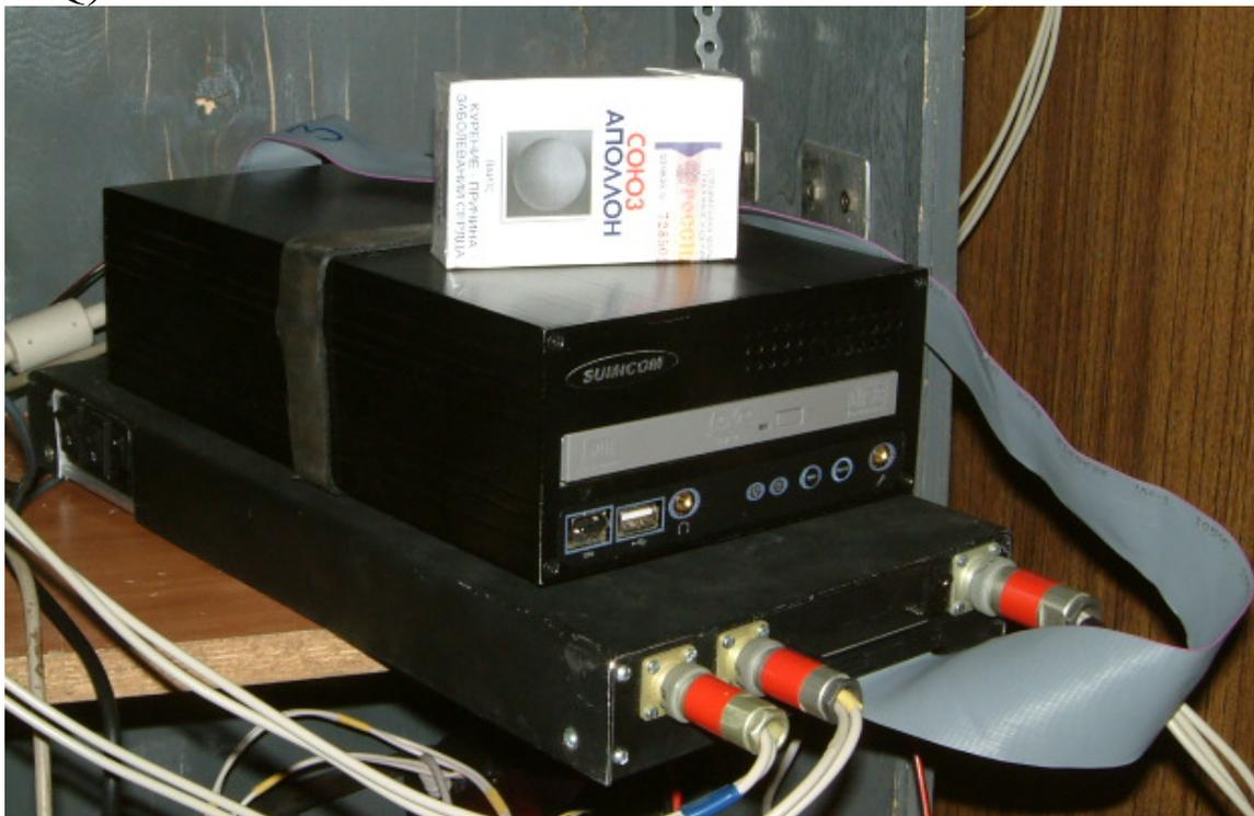
View of interface connected to data acquisition board (16 bit NI DAQ) installed in industrial computer.
