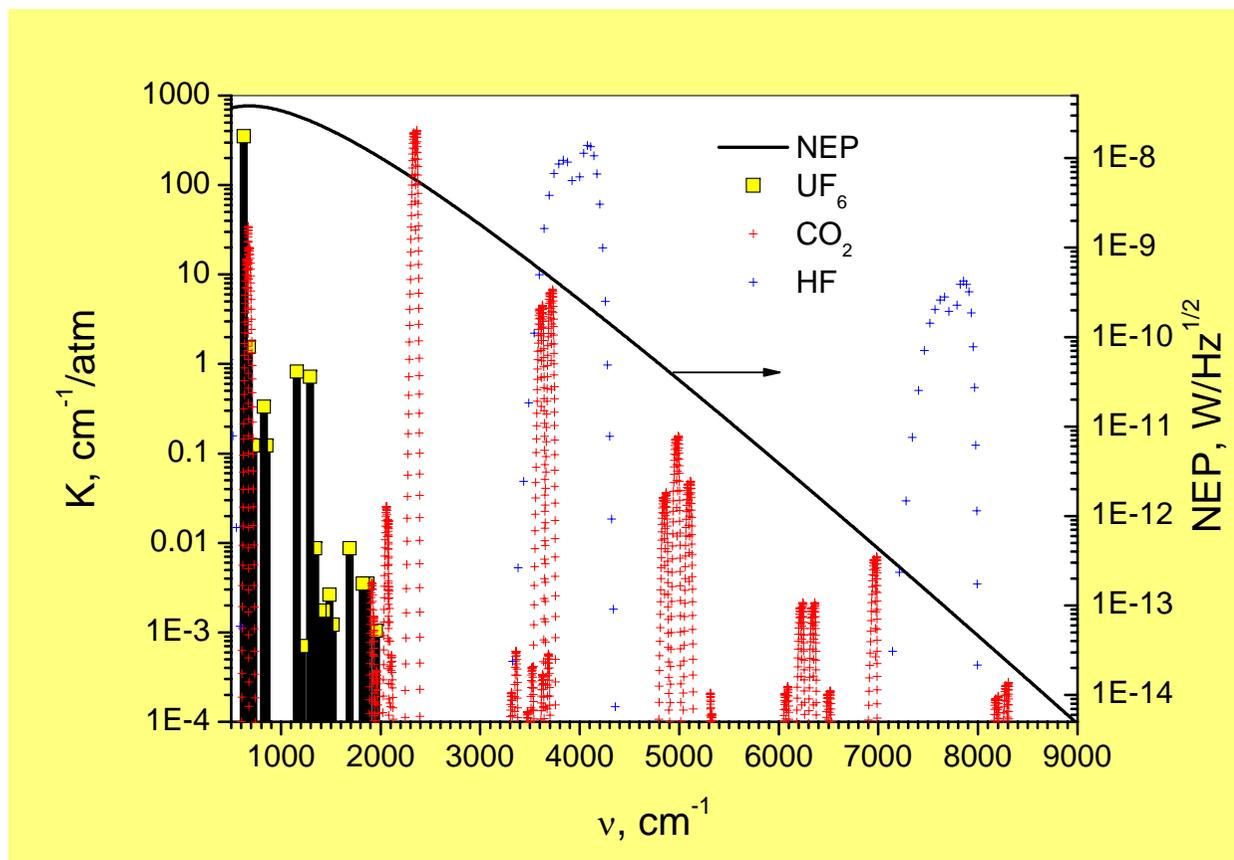
Comparison between absorption spectra of representatives of three molecular groups and photo-diode NEP (Noise Equivalent Power).
