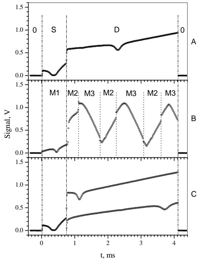
Left - examples of TDLS operation modes; 0 – DL current below threshold, S and D – regions used for stabilization and analytical purposes.
