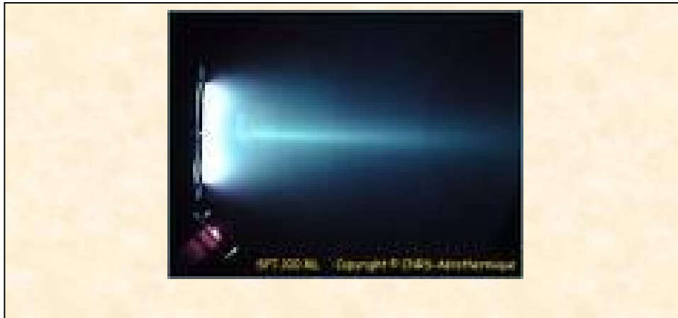
Fig.1 SPT 100 Hall Thruster in operation
