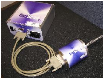
Fig.1 PSI TDLS sensor for fuel tank head space O 2 concentration, the GasScanO 2
