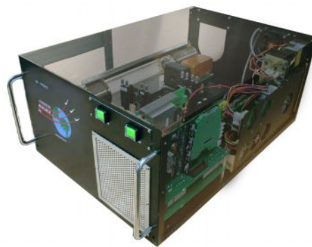
Figure 2. Photograph of the compact ammonia instrument (without covers). Optical module is on the left; electronics module is on the right.
