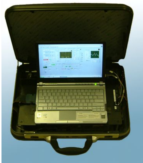
Fig 1. Photo of the compact prototype of the device intended for rapid analysis of trace quantities HF in atmosphere with the use of near-infrared diode lasers (DL) and multi-path cell.
