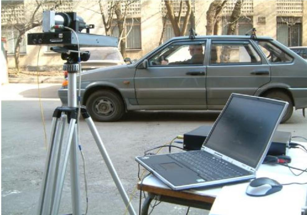
**Field test: remote explosives detection inside moving vehicle.**
