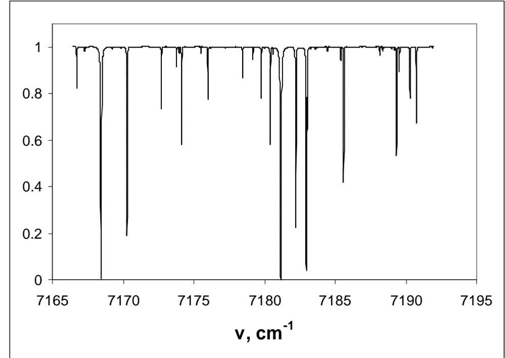
Recorded signal for empty cell (red) and cell filled with sample #1 (black) with broad atmosphere water absorption.
