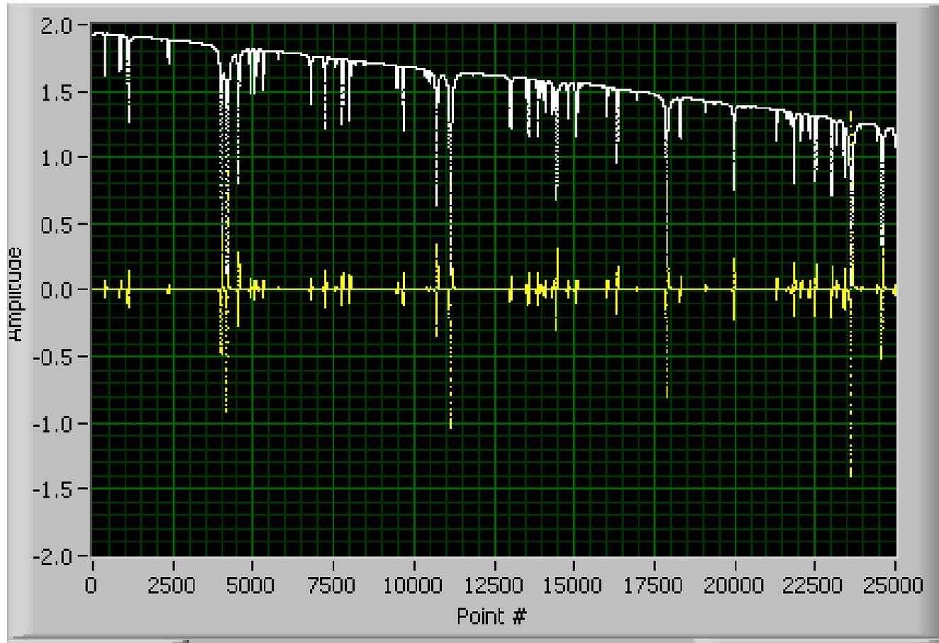
Spectra in broad spectral range were obtained by DL temperature slow changing. DL temperature, DL intensity passed through cell (white), and its logarithmic derivative (yellow) were recorded. Time of recording was 15 min.
