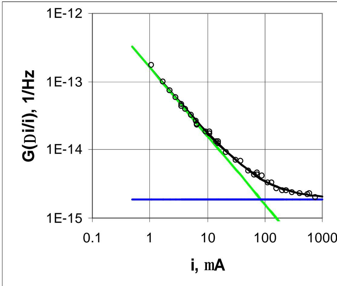
Spectral density of photocurrent relative noise –  $G(Di/i)$  as function of photocurrent value  $i$ .
