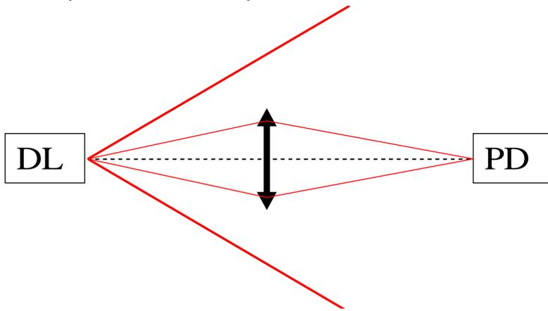
Traditional experimental scheme in TDLS. Part of DL radiation is collected by objective on PD.
