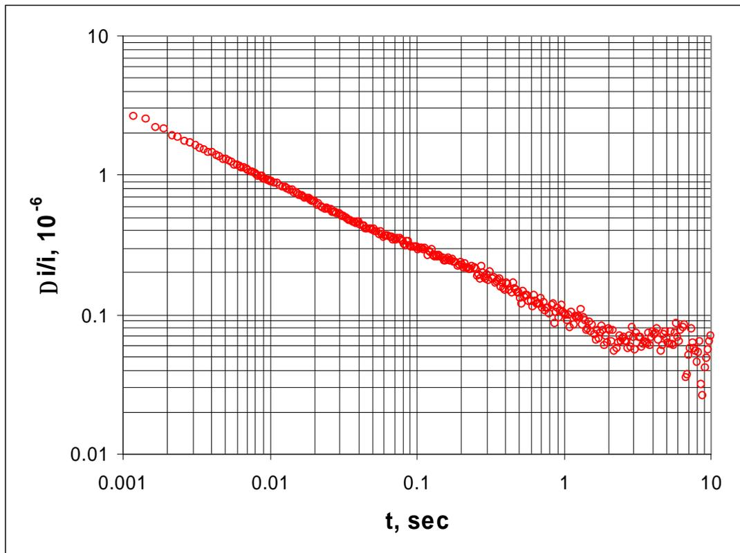
Frequently (in photo-acoustic and ring-down spectroscopy) minimum detectable absorption coefficient is considered. This parameter is equal to  $6 \cdot 10^{-12} \text{ cm}^{-1}$  for our system (Chernin multi-pass cell in use: 0.5 m, 200 passes) and it is comparable with the best known results obtained in Stark spectroscopy.
