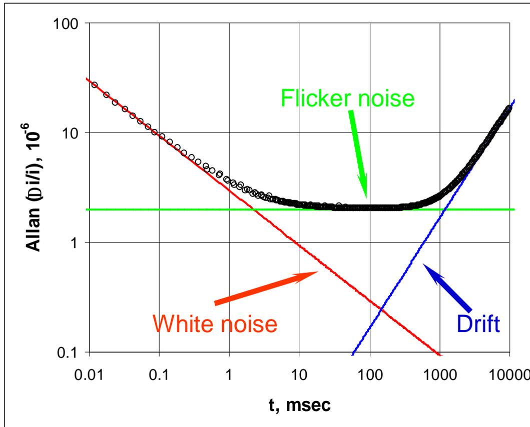
Allan plot of relative photocurrent noise as function of averaging time. There are three main noise types limiting TDLS: white noise (red), Flicker noise (green), and drift (blue). For white noise fundamental limit due to DL quantum noise is achieved. Moreover, white noise can be reduced by increasing of averaging time. Flicker noise and drift can not be reduced by averaging time increase. Physical origins of these noises have to be identified to reduce their influence.
