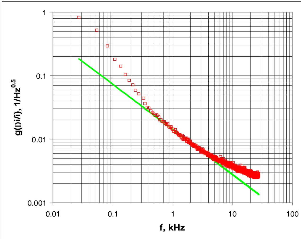
Spectral density of DL frequency noise (excitation current was chosen to detect signal on slope of spectral line). Green line corresponds to  $n = 1.42$ , the same as for intensity noise.
