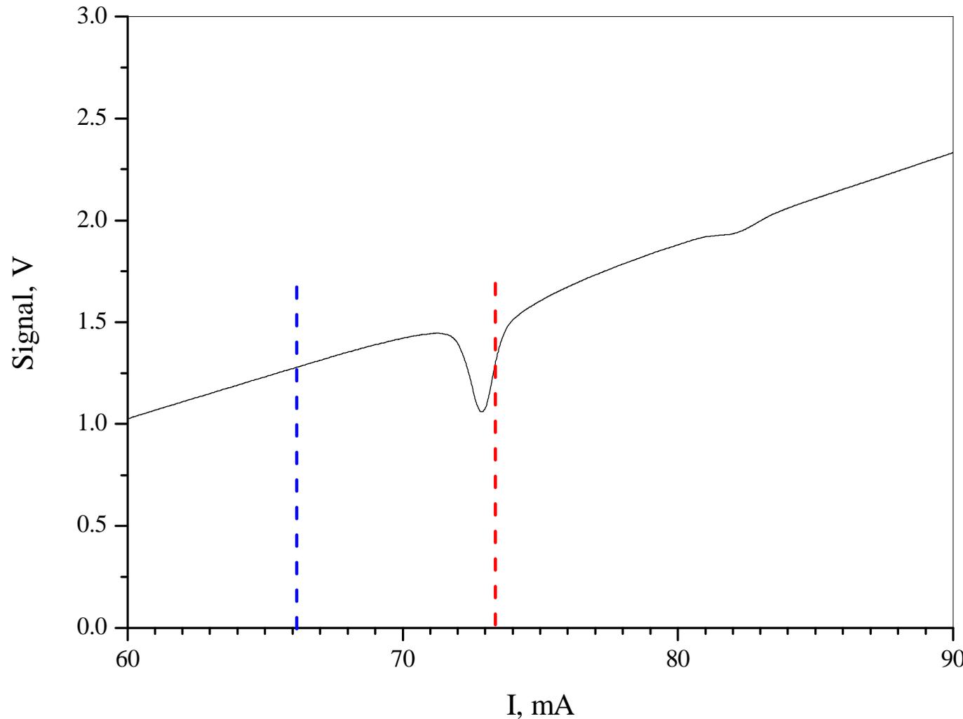
Recorded signal as function of excitation current. Presence of resonant molecular line can be observed. For excitation current out of the line (blue dashed vertical line) DL intensity noise will be measured. For excitation current corresponding to line slope (red dashed vertical line) DL frequency noise will be transformed into intensity one and mainly this noise component will be measured.
