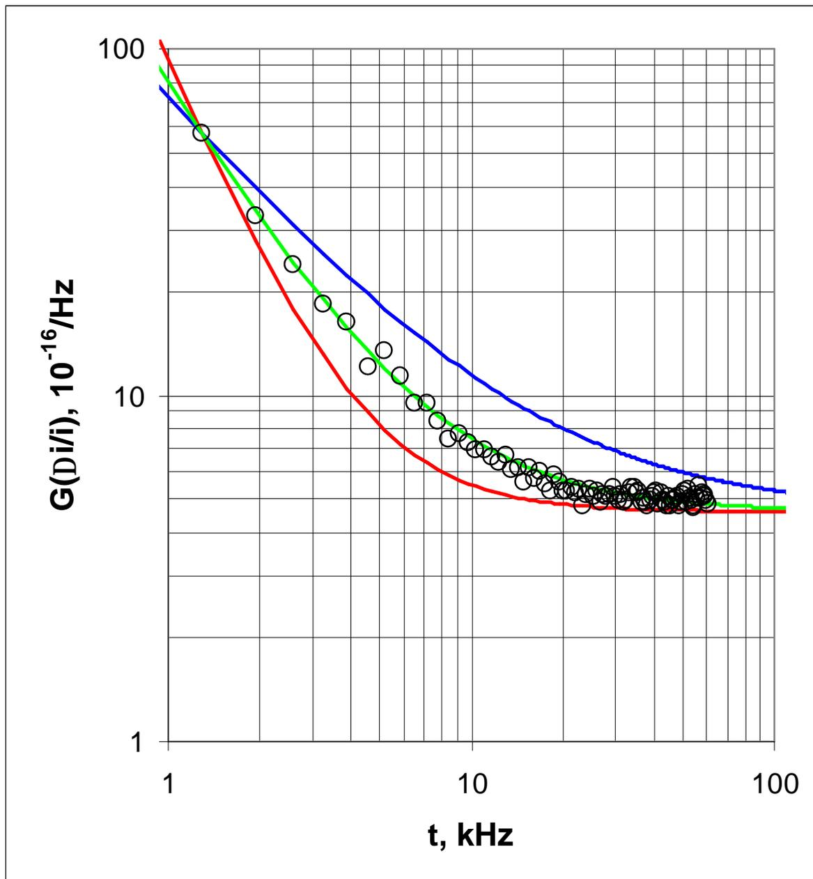
Spectral density  $G$  of relative photocurrent noise (intensity noise, excitation current was out of spectral line).
