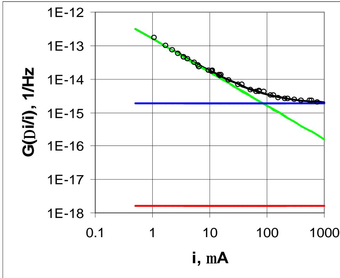
Electrons in PD. Electrons are particles - photocurrent shot noise (green line).
