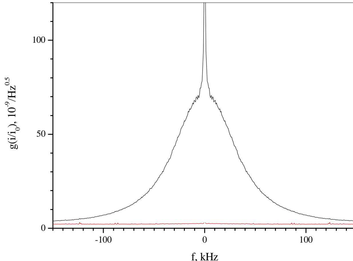
Photocurrent noise spectral density: black - DL on, red - DL off. Broad spectrum feature is determined by DL quantum noise and preamplifier in use (white noise).  $i_0$  corresponds photocurrent recorded for excitation current equal 2 threshold values.
