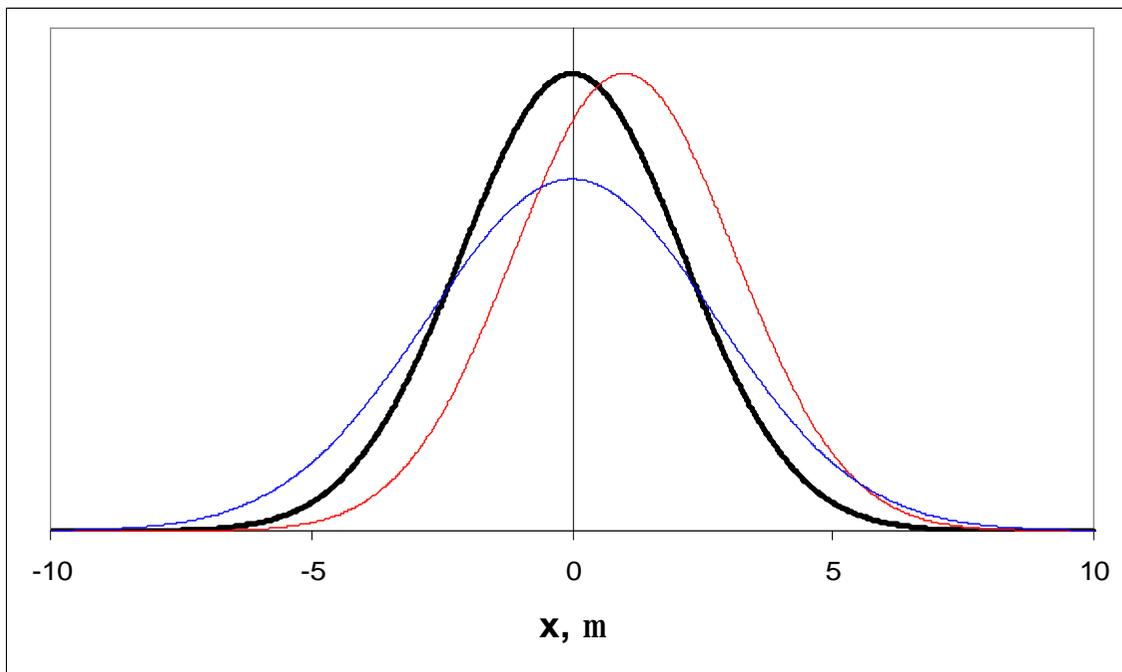
$\Delta x$  describes flicker noise shift of DL near field pattern (red curve).  $\Delta D$  – is the flicker noise pattern width change (blue curve). As excitation current shot noise is negligible, integral below curve has to be constant (**main characteristic of noise under consideration**). Hence, with increase of the pattern width, proper decrease of its maximum has to take place.
