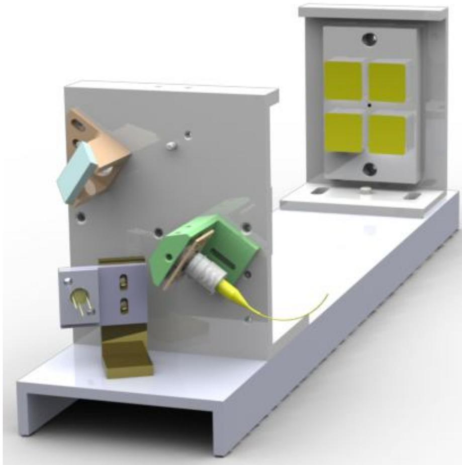
Analytical channel module layout drawing: “Chernin” matrix optical system ( $L = 39$  m), DL fiber input into cell, mirror, and PD to detect DL light from cell.
