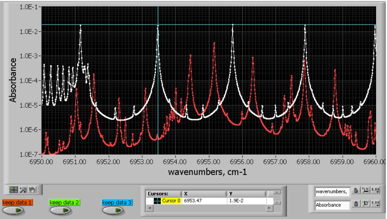
HITRAN 2008 based modeling of CO<sub>2</sub> and H<sub>2</sub>O absorbance in selected spectral range white and red, respectively.
