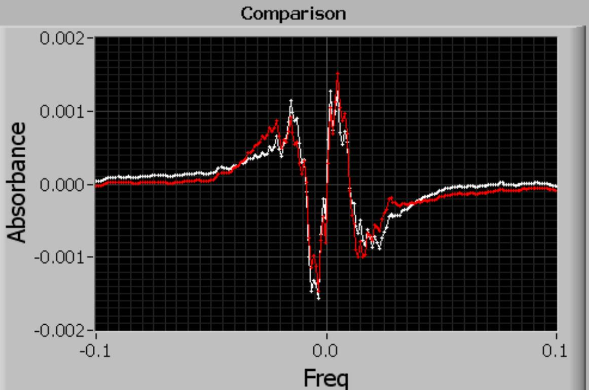
Residual for fitting using hard (red) and soft (white) models. The residual has 3 roots – asymmetry (previous slide and B2).
