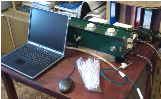
TDL spectrometer - laboratory design
