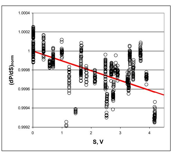
Nonlinearity of all PD and preamplifiers of the spectrometer was calibrated. Example of nonlinearity calibration of analytical cannel PD#4 - 0.023 % (red line).
