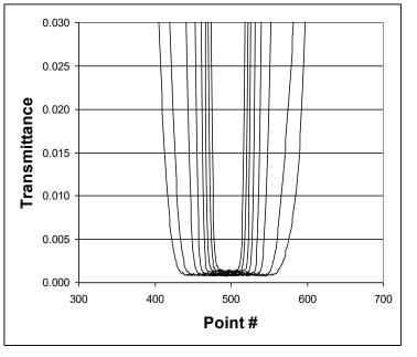
Fragment of spectra presented on previous slide. Optical zero can be easily observed subject of its calibration.
