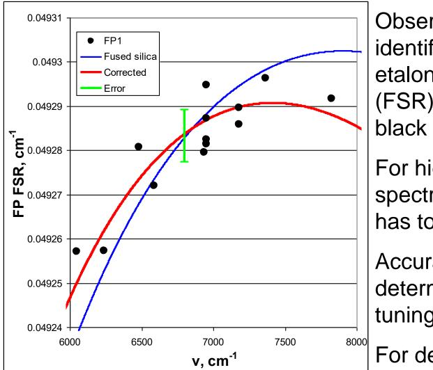
Observed spectral lines were identified using HITRAN and FP etalon Free Spectral Range (FSR) was determined (solid black circles).
