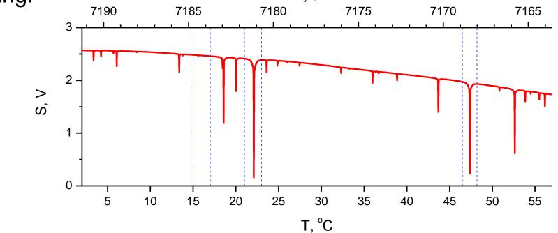
Example of DL calibration with water vapor absorption. After identification of observed lines, analytical spectral ranges can be determined as well as DL temperature to operate in these ranges. In present case three spectral ranges (dashed vertical blue lines) were selected to investigate  $H_2O$  with this DL for different applications.
