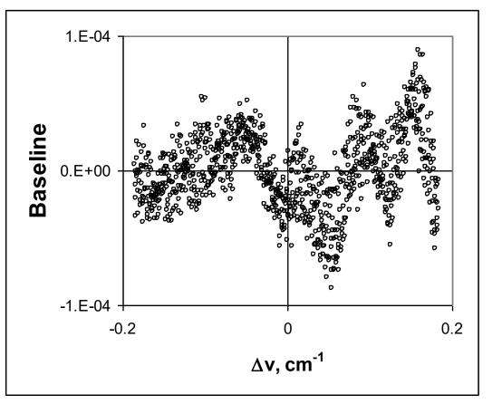
Due to present spectrometer configuration, recorded signals have long term reproducibility. Baseline is difference of empty cell absorbance for signals recorded during time of experiment (20 min).
