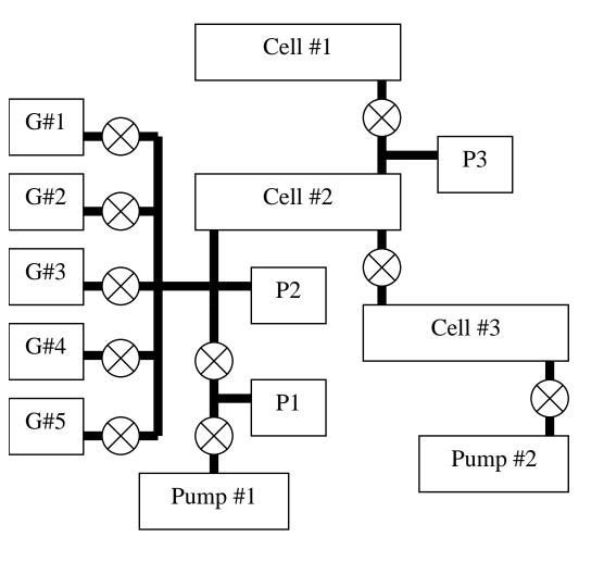
To deal with gas mixtures under investigation vacuum-gas system was developed.
