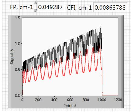
X fiber splitter was used for CFI. To form CFI, two splitter fibers were connected though 10 dB attenuator. CFI FSR (~ 0.00864 cm<sup>-1</sup>) is in agreement with high resolution spectroscopy requirements.
