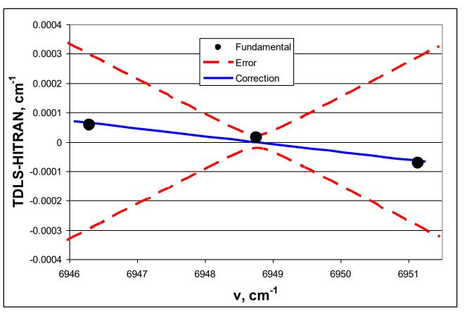
Frequencies of three CO<sub>2</sub> lines of 00031-00001 fundamental band were determined. Solid black circles – difference between present measurements and HITRAN 2012.
