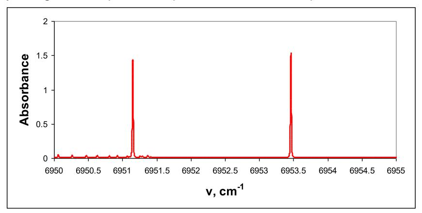
Isolated  $CO_2$  line 6953.467 cm<sup>-1</sup> (P20e of 00031-00001 fundamental band) was selected as analytical one for this test.
