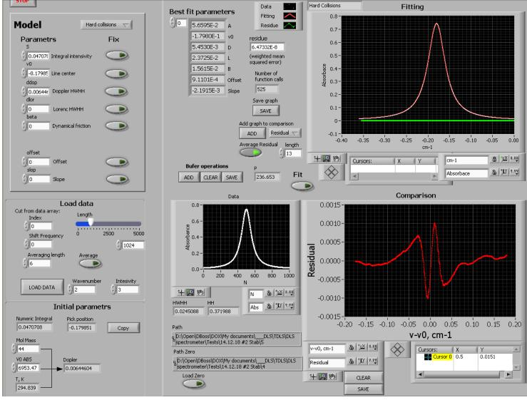
The program provides high accurate experimental spectra fitting (in present case  $CO_2$  line for 236.65 mBar) using Soft and Hard models of Doppler profile. Fitting parameters: A, v0, D, L, B, offset  $\mu$  slope – baseline and its slope, respectively.
