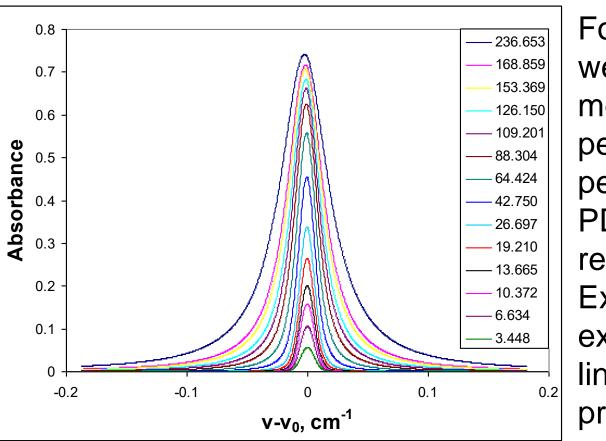
For each pressure, two spectra were recorded. Eight measurement series were performed during 20 days period using different cells and PDs to check reproducibility of results obtained. Example of one of the series experimental results. Here  $v_0$  is line center position for zero pressure.
