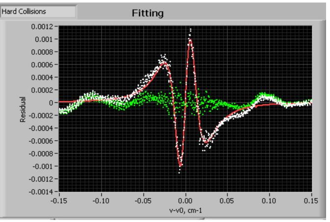
This asymmetry (red curve) can be calculated using line parameters determined experimentally and independently (C1).
