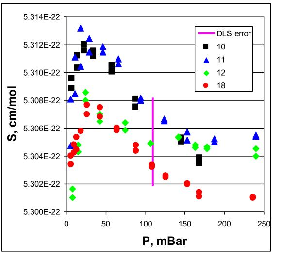
More accurate integral intensity measurements were obtained with cell #2 subject of more accurate the cell length and pressure measurements and Hard model.
