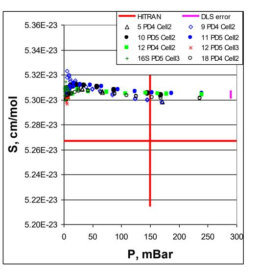
Horizontal red constant is HITRAN integral intensity for analytical line. HITRAN accuracy estimation for this line is 1 - 2 %. Vertical red line corresponds 1 %. Our data can confirm HITRAN accuracy estimations. The reverse is not valid.
