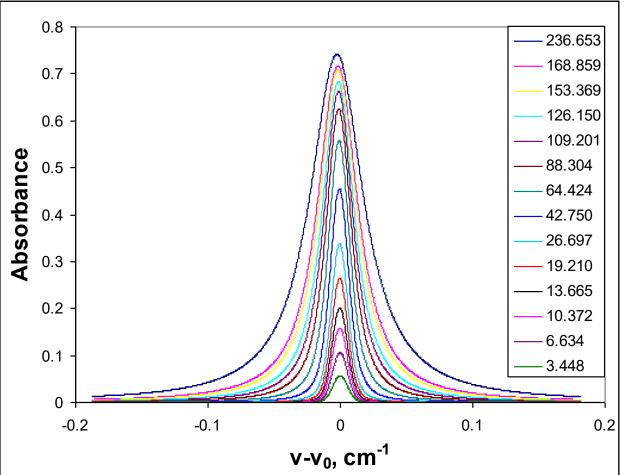
For each pressure, two spectra were obtained. Eight measurement series were performed during 20 days period using different cells and PDs. The purpose of this procedure was to check results reproducibility.
