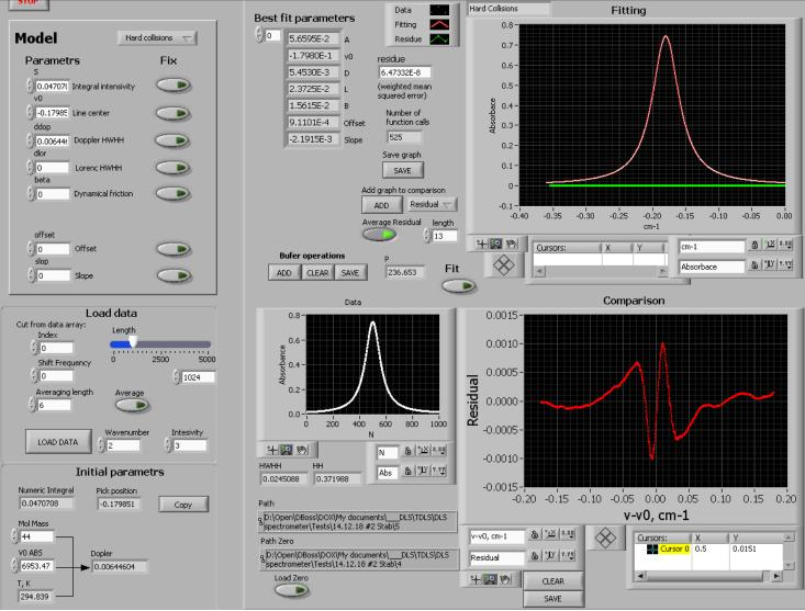
The program provides high accurate experimental spectra fitting (in present case  $CO_2$  line for 236.65 mBar) using Soft and Hard models of Doppler profile. Fitting parameters: A [cm<sup>-1</sup>] – absorbance integral, v0 – line center, D – Doppler width, L – Lorentz width, B – narrowing, offset – baseline. All parameters can be fixed or included in fitting. For present precision no more than 5 parameters can be used (A2).
