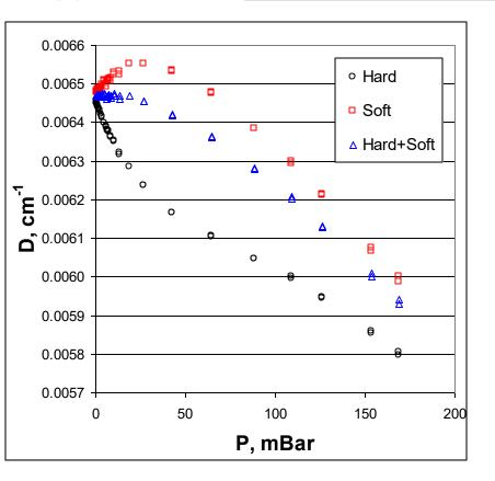
Significant difference can be observed. D is constant below 20 mBar for Soft+Hard.
