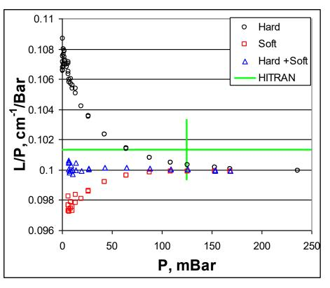
Significant difference (~10%) between models can be observed for small P. Using <u>Hard+Soft = Hard<sup>0.3\*</sup>Soft<sup>0.7</sup></u> final values were calculated. Final values are constant for whole pressure range under investigation. Green constant – HITRAN (accuracy 1-2 %), green bar – 2 %. TDLS accuracy – symbols height.
