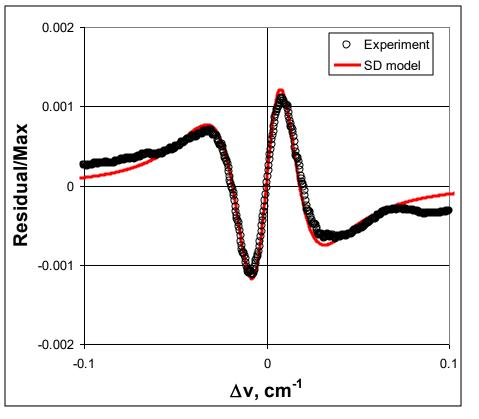
Experiment (black circles) – analytical  $CO_2$  line residual for 236.65 mBar (slide 5). It is asymmetry due to speed dependence.
