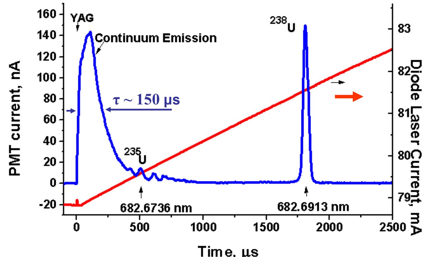
DL wavelength scanning rate  $\sim 0.016 \text{ pm}/\mu\text{s}$
