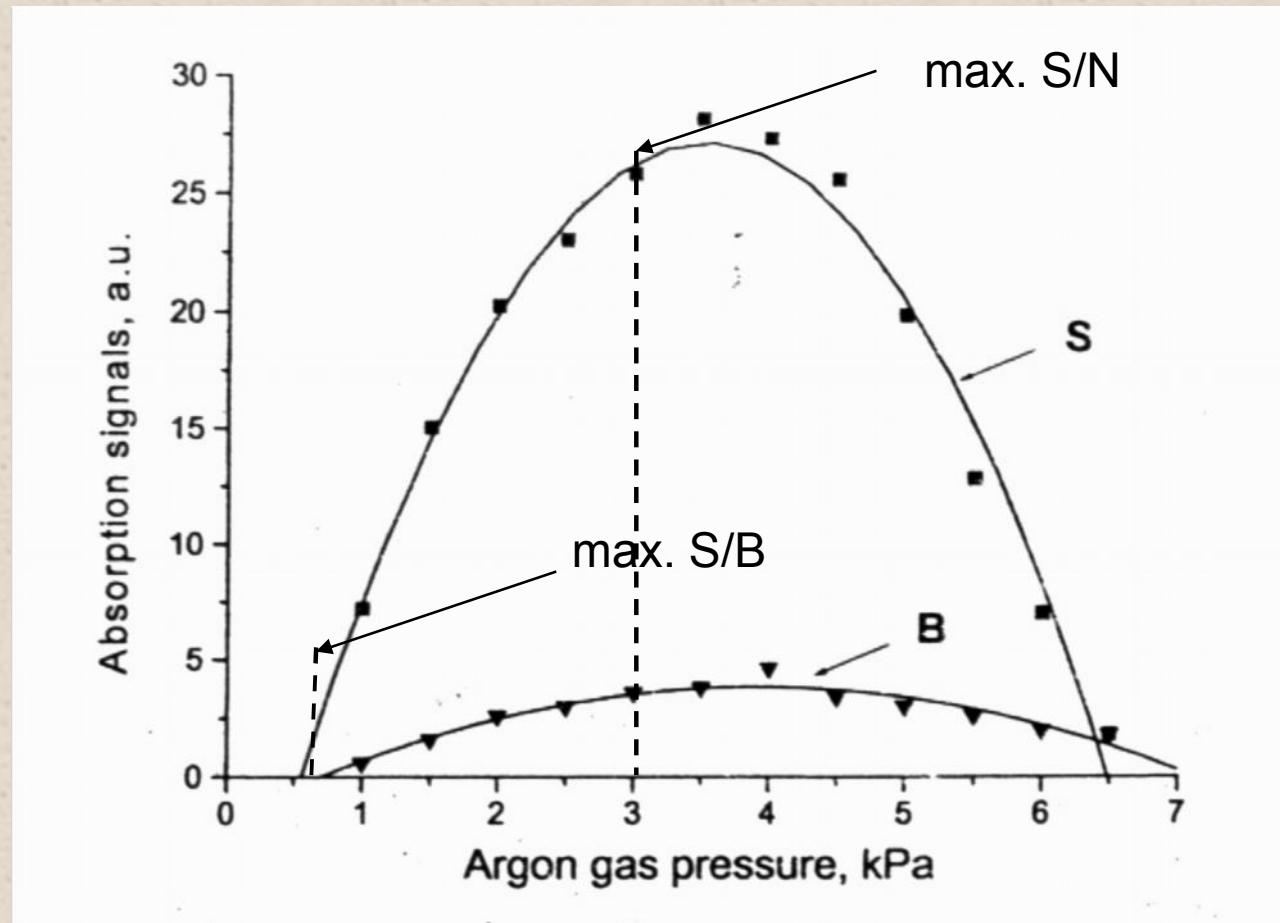
S – background corrected  $^{235}\text{U}$  net absorption signal
